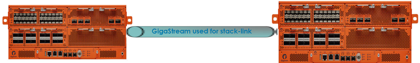
Figure 4 Daisy-Chain Configuration using GigaStream for Stack-link
